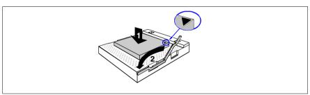
Figure 13: Installing the new processor
